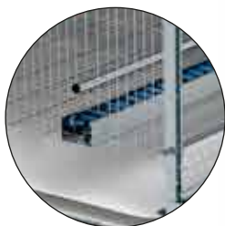
Flat chain feeding system on each tier
